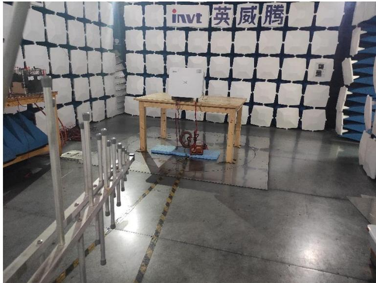
**Test Setup (30MHz-1GHz)**
