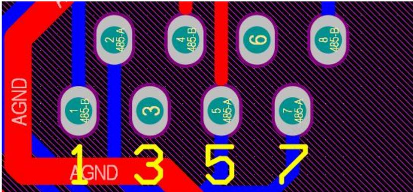
Definition of RJ45 Port Pin for parallel 1.
