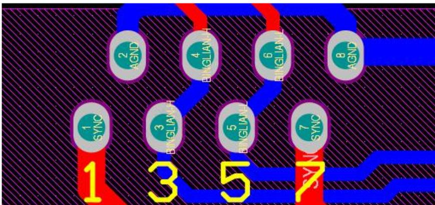
Definition of RJ45 Port Pin for parallel 2.
