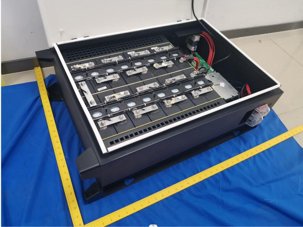
Figure 5 Inside view of battery
