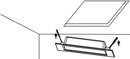
3. Hold the two clips back against the panel light and push it into the hole. Allow the springs to pull the light up to the ceiling.
