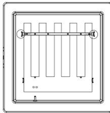
4. Press the buckle outwards, remove the aluminum substrate pressing strip from the bayonet, and remove the pressing strip. This step is only required for 24W panel light, other items are not required.
