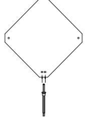
6. Take out two-cord cable (wire diameter 18-22AWG) and insert it into the plug-in terminal. Connect the external power supply for testing.
