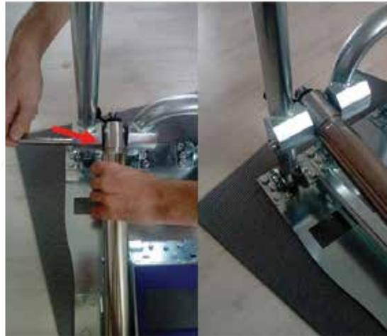
**Figure 33 - Inserting the safety pin**
