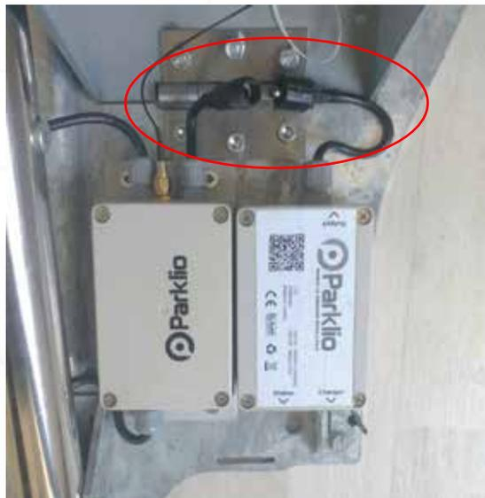
**Figure 13 - Connection of the power supply**
