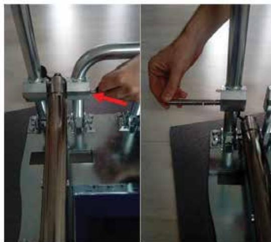
**Figure 34 - Removing the safety pin**
